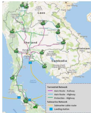
FIBER OPTIC NETWORK ALONG RAILWAY - SRT
